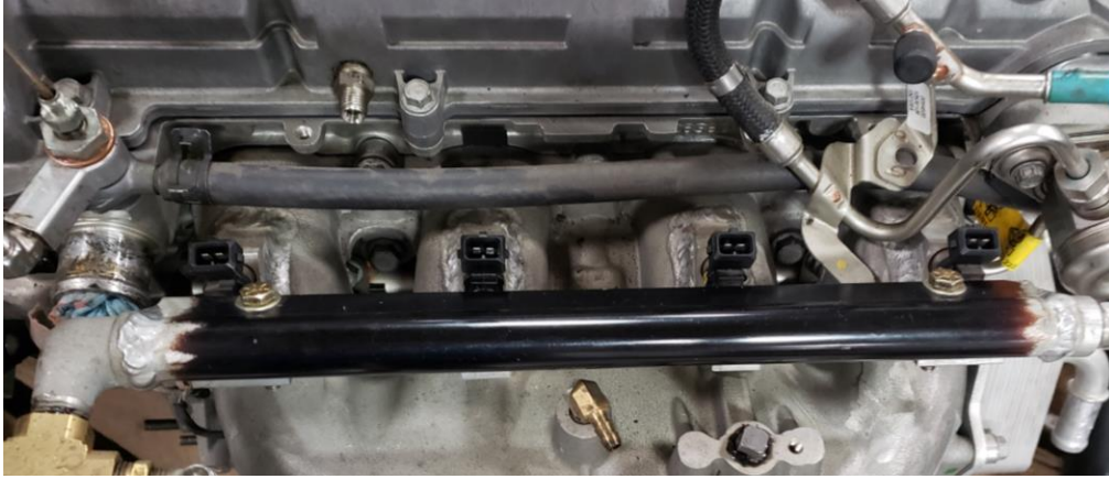
Figure 9 Water injection manifold, water rail and injectors
